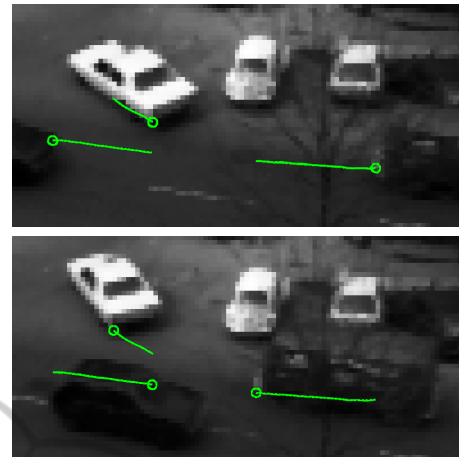
Figure 6: Motion results given as trajectories, with the position ( circle ) of a characteristic point on the first frame ( top ) or the last one ( bottom ).
