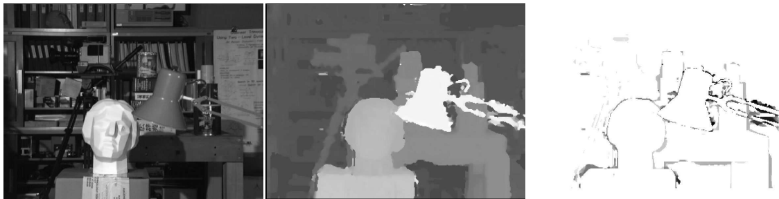
Figure 1: Performance of the plane-sweep algorithm for the data set Tsukuba with the aggregation function A3 and the interaction set I1. On the left, the reference image. In the middle, the output depth map. On the right, absolute deviations of disparity are shown. All pixels with deviations below one pixel are marked white.
