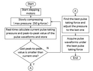
Figure 6: Searching process of the best pulse taking force.
