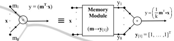
Figure 1: Implementation of an elementary memory module by the octonionic module.
