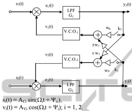
Figure 3: The oscillating (PLL) neuron model.
