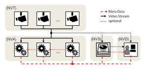
Figure 2: ONVIF-based network architecture.
