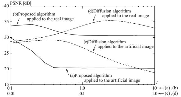
Figure 5: Image denoising processes evaluated by the measure PSNR. Curves (a) and (b) show results of the proposed algorithm applied to the artificial and real images (see Figs 3 and 4). Curves (c) and (d) show results of the diffusion algorithm applied to the same artificial and real images; the algorithm achieved the best performance at  $t = 0.04$  on the artificial image, and at  $t = 0.24$  on the real image. Note that a time scale for (a) and (b) is different from that for (c) and (d).
