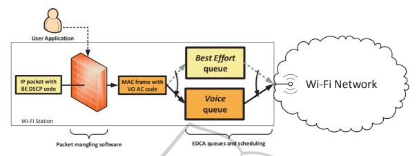
Figure 1: Example of a traffic remapping attack performed by a user of a Wi-Fi station taking advantage of traffic differentiation provided by the enhanced distributed channel access (EDCA) function of IEEE 802.11.
