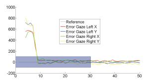
Figure 5: This figure depicted the error (gaze coordinate minus the target coordinate) as a function of time. In this figure the gray rectangle enclose the first 0.75 seconds not used for the analysis because it is considered the time required to fix the gaze in the target displayed.
