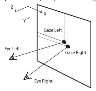
Figure 3: This figure depicted the gaze for each eye projected to the screen as a red and blue line. Also are depicted the points of intersection between the gaze and the screen (red and blue circles). Coordinates origin is the upper left corner of the screen.
