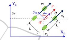
Figure 1: Kinematics of the Pioneer P3-AT mobile robot.
