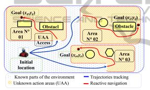
Figure 3: Descriptive diagram of the navigation approach.
