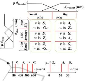
Figure 6: Fuzzy rules basis and outputs sets for the obstacles avoidance controller.
