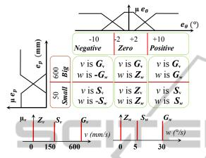
Figure 5: Fuzzy rules basis and outputs sets for the trajectory tracking and goal seeker controller.
