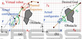
Figure 2: (a) Trajectory tracking problem based on virtual approach, (b) reactive navigation problem in unknown environment.
