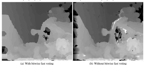
Figure 8: Comparison of the results with and without bitwise voting for stereo methods using fixed square aggregation windows. The results are clearly better when applying bitwise voting. This demonstrates that this method is not only applicable to the aggregation windows described above.
