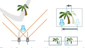
Figure 1: Concept of stereo vision. A scene is captured using 2 rectified cameras. Stereo matching attempts to estimate the apparent movement of the objects across the images. A large apparent movement (i.e. parallax) corresponds to close objects (a low depth value) and vice versa.
