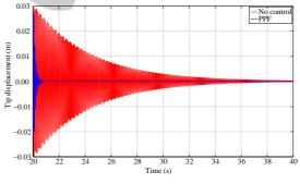
Figure 6: Tip displacement vs. time with and without control.
