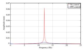
Figure 7: The FFT spectrum of the smart beam.
