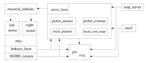
Figure 3: System interaction methods.
