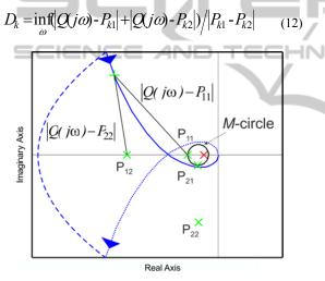
Figure 2: Calculation of  $D_1$  with checkpoints  $P_{11}$ , and  $P_{12}$ .
