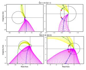
Figure 4: Nyquist-array of the designed loops.
