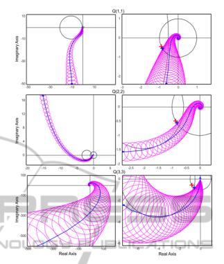
Figure 5: Nyquist-array of the designed loops.
