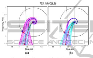
Figure 6: Nyquist-array of the designed loops.
