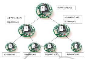
Fig. 2. Example of Integrity Preserving Secure Data Aggregation.
