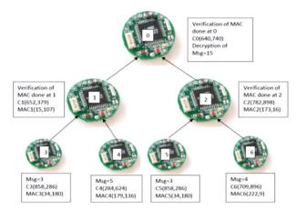
Fig. 3. Example of Privacy and Integrity Preserving Secure Data Aggregation.
