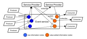
Figure 2: Crowdsourcing model based on a pubsub scheme (Szabó et al., 2013).
