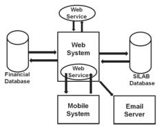
Figure 2: SILAB architecture.
