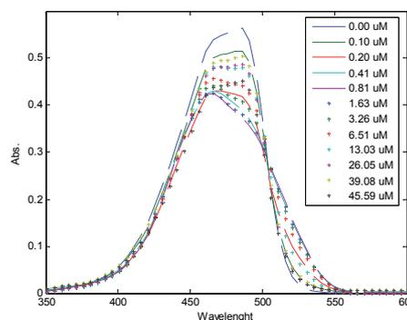
Figure 3: Absorption spectra of 10uM BO21 at various concentrations of heparin.
