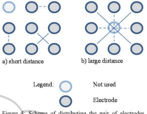
Figure 4: Scheme of distributing the pair of electrodes (bipolar) oriented every 45° with different distances between electrodes. b) Short distance b) Large distance.
