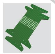
Figure 11: Prototype of flexible sensor array for detection of motor unit activity.
