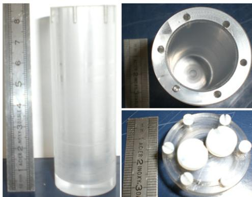
Figure 3:  $\mu$ SPC phantom body.
