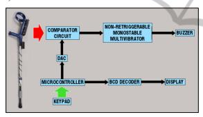
Figure 1: Block diagram of the biofeedback module, including the instrumented Lofstrand crutch.
