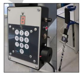
Figure 4: Biofeedback module and the final version of instrumented Lofstrand crutch.
