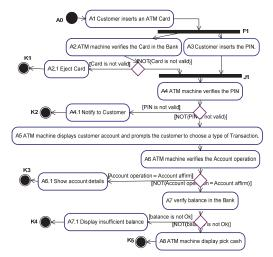
Figure 3: Activity Diag of ATM system balance withdraw.
