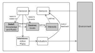
Figure 4: Internal Architecture of a CAKMAS Agent.
