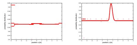
Figure 3: Influence of the position in the x- and z-axis on the result of the probability distribution. On the left graph it can be seen, that the position in the x direction has no real influence on the result of the pre-classification. In contrast, the height of the object influences strongly their classification
