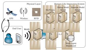
Figure 3: Physical architecture for the system.
