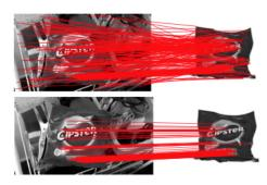
Figure 8: The images show the matches with (lower) and without (upper) RANSAC.
