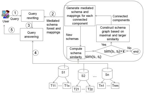
Figure 2: A query system with hierarchical mediated schemas.
