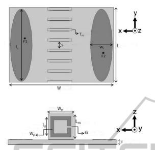
Figure 1: Two-element antenna array based on elliptical patch radiating elements with MNG. Top view (top) and side view (bottom).
