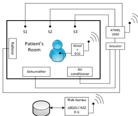
Figure 2: Indoor Monitoring System Architecture.
