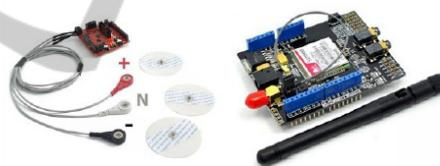
Figure 1: ECG with the acquisition shield (left) and the GPRS shield for data communication (right) used in the implementation.
