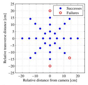
Figure 7: Results for pick with variation in position relative to position used during teaching. The figure shows the tabletop from above, and the camera position was to the left. The pick operation succeeded for all positions with variations up to 15 cm. For errors of 20 cm, the pick operation failed in 3 of 8 cases.
