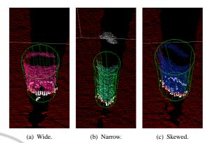
Figure 8: Rotations of the most deformed cylinder from Figure 6(a). For the wide and skewed orientations, a containing cylinder is fitted successfully. For the narrow orientation, the containing cylinder is only fitted to the frontal part of the physical cylinder.
