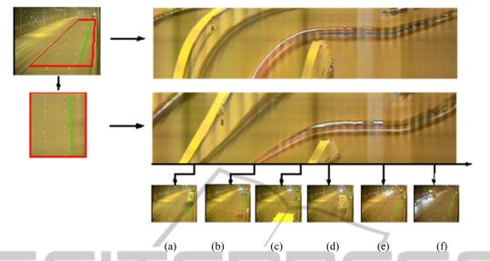
Figure 6: Top: original image and the TSI corresponding to the green line. The red square is used for the perspective compensation. Middle TSI after perspective correction. Bottom: original images illustrating the successive events.
