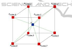
Figure 7: Interpolation of intermediary voxels. Red filled squares represent voxels from the oversampled voxel space while the blue squares inside the cube represents a voxel from the normal voxel space. Green dashed lines represent the distance from the center of the voxel *P* to one of the cube corner voxels.
