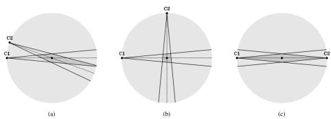
Figure 4: Overlapping area for an angle of  $20^{\circ}$ ,  $90^{\circ}$  and  $180^{\circ}$  between camera C1 and C2 for a certain voxel in space. We see that the overlapping area (dark gray area) presents respectively 2.99%, 0.75% and 4.08% of the marked space (lightgray area). We notice an angle of  $90^{\circ}$  reduces the overlapping area significantly.
