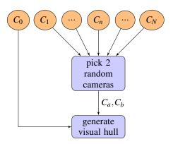
Figure 1: Flowchart to determine which voxels are not occluded for camera  $C_0$ . Two cameras are randomly picked from the list and we calculate the visual hull from their masks together with the mask of camera  $C_0$  from which we try to determine the occlusion map. Since camera  $C_0$  contributes to the visual hull the result is a shape which is not occluded for these cameras.
