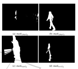
Figure 3: (3(a)) The mask of the camera  $C_0$  for which occlusion is checked. (3(b)) The mask of one of the randomly chosen camera views  $C_a$  (3(c)). The reprojected image of the visual hull generated only by mask (3(a)). (3(d)) The occluded part shown in white, which is combined with two other cameras to calculate a visual hull and update the occlusion map.
