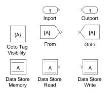
Figure 1: Additional Simulink data flow mechanisms.
