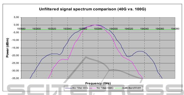
Figure 3: Unfiltered 40 G and 100 G signal spectrum.
