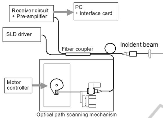
Figure 3: Portable OCT scanner.
