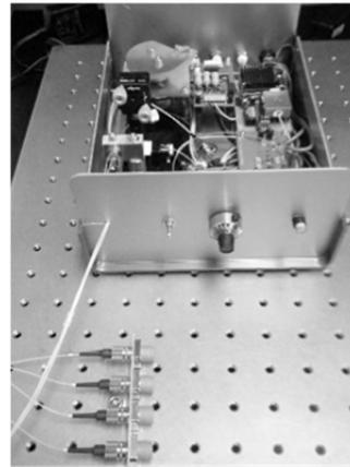
Figure 9: Multi-channel probes on a portable OCT.
