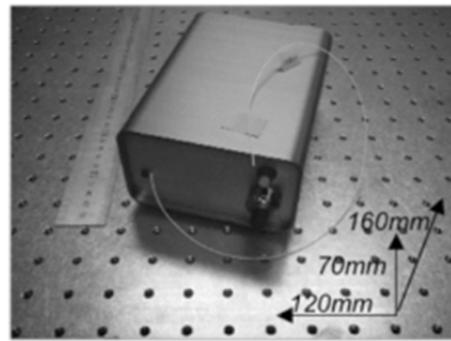
Figure 4: Portable OCT scanner.
