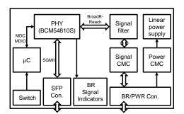
Figure 1: Block diagram of a Technica/tinytron optical Ethernet-to-BroadR-Reach media converter.
