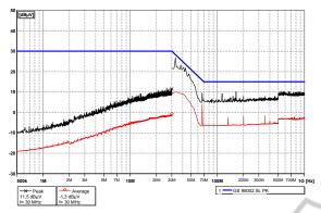
Figure 4: Result of the emission measurement. Blue: Limit line from GS 95002; Black: Peak detector result; Red: Average detector result.
