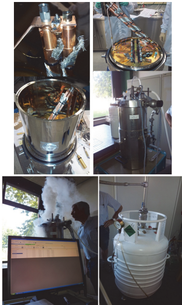
Figure 11: Photographs of cryogenic test set-up and Helium facility (SRON) for controlled 40K cycle tests.
