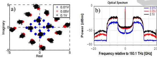
Figure 6: (a) Larger drive amplitude increases the distance between symbols but (b) outside of the OFDM spectrum the noise level also increases.
