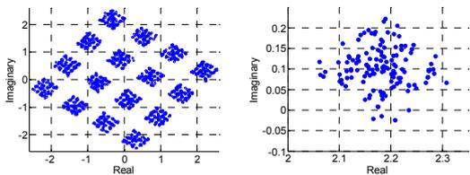
Figure 8: (a) Symbol deviation caused by SPM and FWM. (b). Only FWM caused symbol spread at one symbol.
