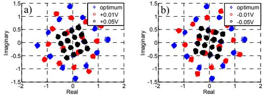
Figure 4: (a) Constellation turns right, if the bias error is positive and it turns left (b) when the bias changes negatively.
