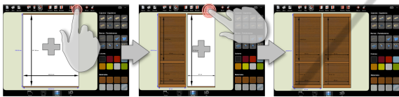
Figure 3: Door creation process. Each single tap on the associated button triggers the calculations needed to parametrically define a new door and change the position and scale parameters of previously created doors.
