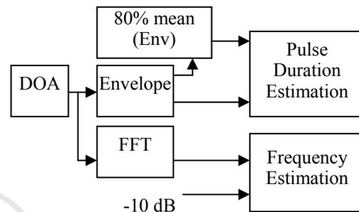
Figure 6: The block-scheme of sound parameters estimation
