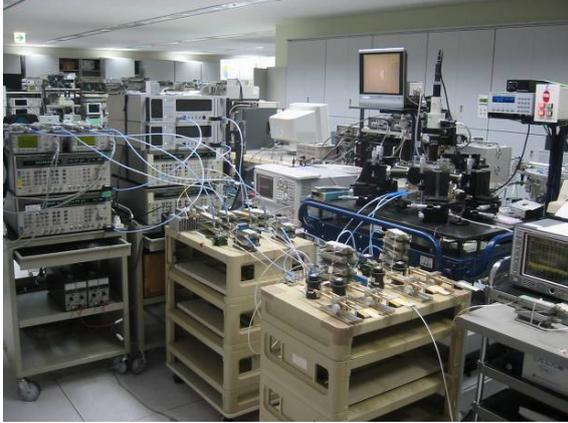
Figure 4: Experimental configuration for IMD measurement.
