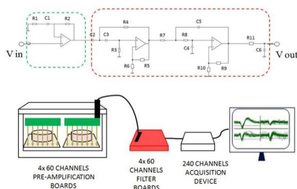
Figure 2: Schematic of the custom front-end circuitry (top) and assembly of the boards (bottom).
