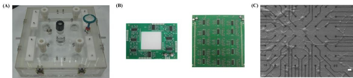
Figure 3: (A) Picture of the realized environmental chamber. (B) Assembled electronic boards for the internal pre-amplifier stage (left) and external filter stage (right). (C) Inverted microscope image of a neuronal culture grown on a MEA taken from the chamber (bar scale 10 μm).
