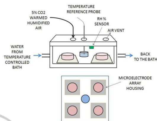
Figure 1: Schematic representation of the environmental chamber (top) and top view of MEAs housings (bottom).
