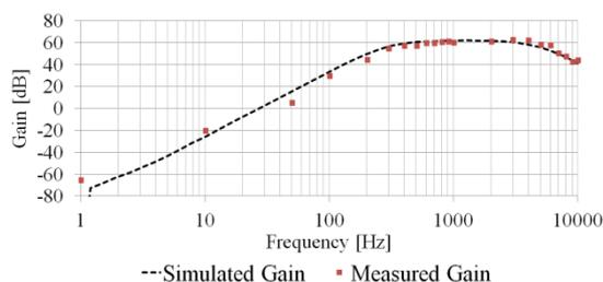
Figure 6: Comparison between the simulated gain and the measured one (pre-amplifiers + filter boards).
