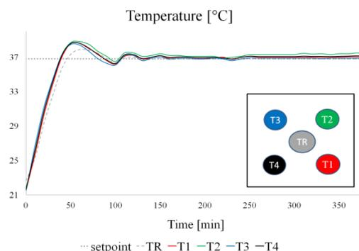
Figure 4: Temperature time course measured at the reference well (dotted line) and at the four MEAs allocations (T1-T4). The insert is a top view of the temperature measurement points.
