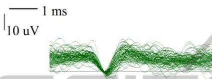
Figure 7: Overlapped neuronal spikes recorded from a MEA channel inside the environmental chamber.
