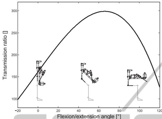
Figure 3: Transmission ratio as a function of the angle in the sagittal plane. In the walking range the transmission ratio is smaller. During standing up, the maximum torque is required when the angle is around 70°. The orthosis has its maximum transmission ratio in this range.
