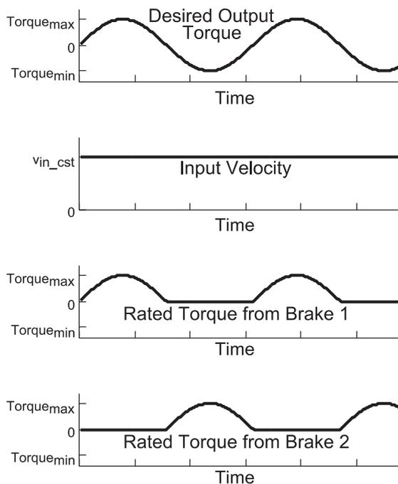
Figure 7: Graph showing the control inputs of the brakes to generate a sinusoidal torque. The velocity source does not need to adapt to the changes. In order to limit losses the brakes should not provide torque at the same time. For a positive output torque, the first brake will be engaged.
