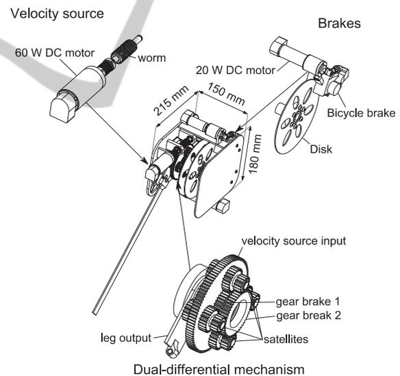
Figure 6: Hip orthosis with a double-differential actuation. The different components which constitute the mechanism are a velocity source (composed by DC motor and a worm gear), two disk brakes and the dual-differential mechanism.
