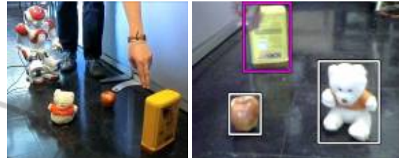
Figure 11: Experimental setup showing the tutor pointing a yellow chocolate box which has been seen, interpreted and learned (by the robot) in term of colors then asking the robot to describe the chosen object (lower left-side) and the ground truth detected objects as the robot perceives them (lower right-side).
