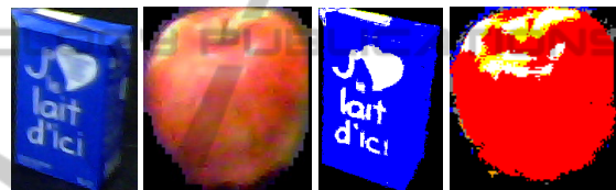
Figure 12: Two objects extracted from robot's surroundings. Right: the original image, left: features interpreted. For the “apple”, the robot’s given description was “the object is red”. For the box, the description was “the object is blue and white”.
