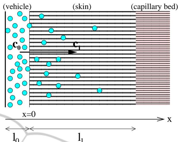
Figure 2: Cross-section of the vehicle and the skin layers. Due to an initial difference of unbounded concentrations  $c_0$  and  $c_1$ , a mass flux is established at the interface  $x = 0$  and drug diffuses through the skin. At  $x = l_1$  the skin-receptor (capillary) is set. Figure not to scale.
