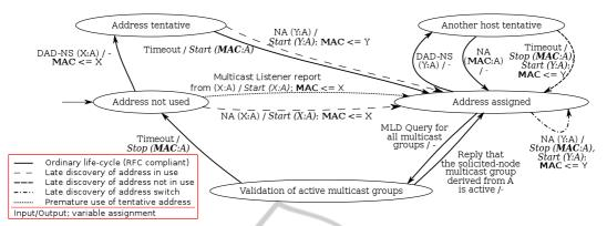
Figure 1: The life-cycle of an IPv6 address A can be monitored by the Mealy FSM extended by the variable **MAC** to store the MAC address of the interface that currently uses A. Binding between MAC address X and A is denoted as (X:A).
