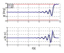
Figure 6: Comparison of q(t) and  $\tau_{\text{max}}$  calculated by using CoV and Reversed Falling Trajectory (RFT).
