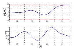
Figure 4: Minimal energy trajectory q(t) and control torque  $\tau(t)$  corresponding to lifting time  $t_f = 4[s]$ .
