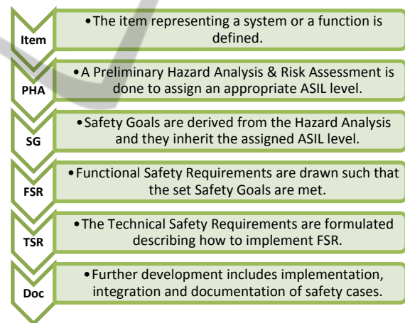
Figure 4: Overview of ISO-26262 safety case & argumentation process.
