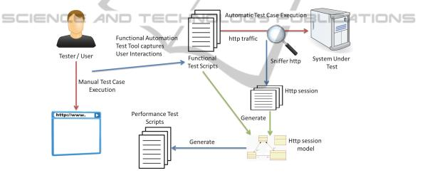
Fig. 3. Scripts generation proposal for performance tests.
