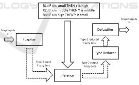
Figure 1: Type-2 Fuzzy Inference System block diagram.
