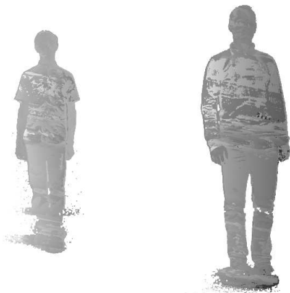
Figure 8: Depth map with a uniform depth plane distribution. A high number of planes (256) is used.
